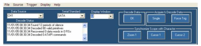
Use the **Data Source** drop-down list to select your data source. Data sources can be Channels 1-4, Math 1-4, Ref 1-4, or File. Selecting File allows you to browse for waveforms stored in .wfm format. If your data source contains FastFrame data, then an additional control appears (to select the frame). Enter the frame number in the Frame control to navigate to a specific frame for analysis.
